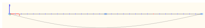
Amplitude values of the deflection \eta_2 in the cross-section of the beam with the attached mass not subjected to the shear force and the deformed models at the respective time points ( m ). Frequency of the harmonic exciting force \omega_5 = 0.95 \cdot p_2
