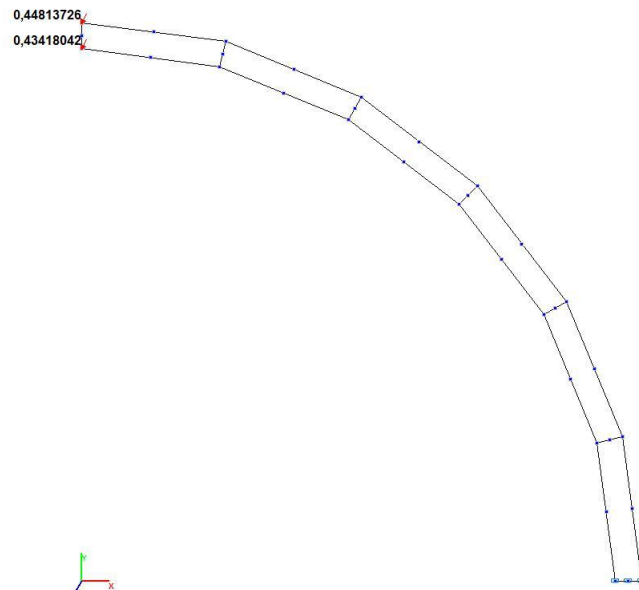
Model 7. Values of the transverse displacements Y, Z of the free end of the curvilinear cantilever beam (m, m)
