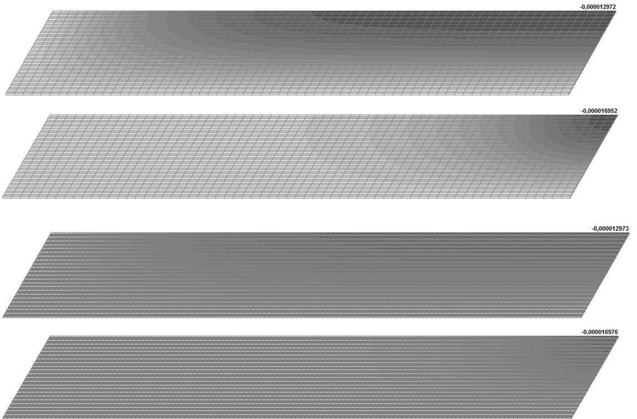
Model 6. Values of the transverse displacements in the center of the simply supported rectangular plate w_q and w_P (m, m)
