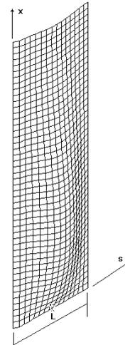
It was assumed that the actual surface deviated from the perfect cylinder with the radius 19950 mm could be described by this equation in the cylindrical coordinate system:
