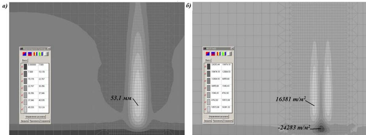
Figure 5: Results of a nonlinear analysis in the area 1: (a) displacements; (b) annular stresses
