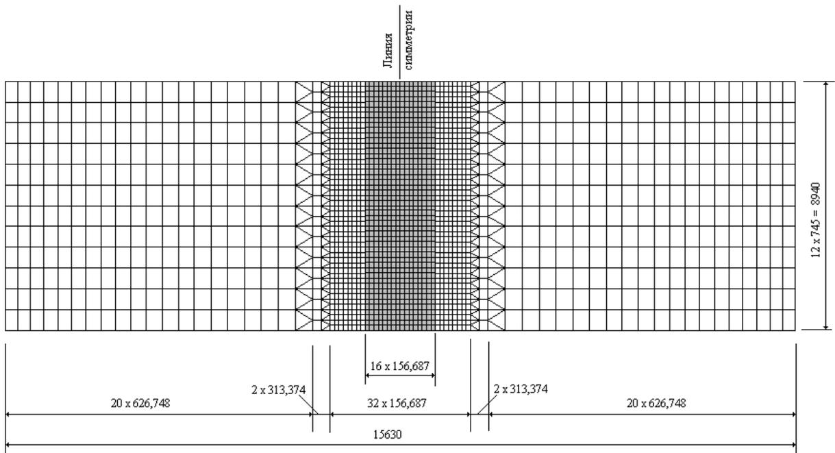
Figure 1: The finite element mesh evolved (the reinforced area is marked)
