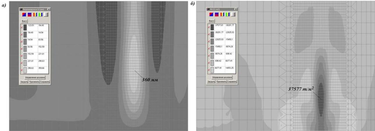
Figure 4: Results of the linear analysis in the area 1: (a) displacements; (b) annular stresses
