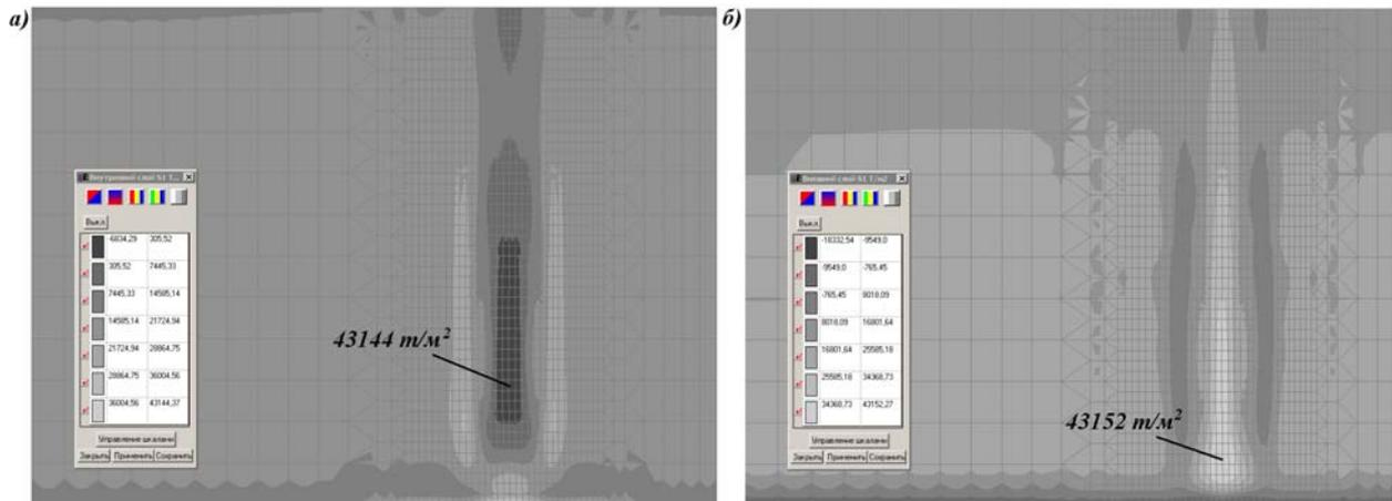
Figure 7: Equivalent stresses in the area 1: (a) in the interior layer; (b) in the exterior layer
