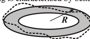
The buckling out of the plane of the ring is characterized by bending displacements that are perpendicular to this plane.
