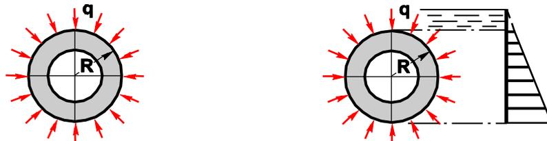
The study is focused on the critical load that leads to the buckling of the ring in its plane or out of its plane.
