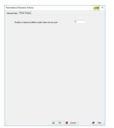
The only characteristic necessary for performing the modal analysis, the number of natural oscillation modes taken into account, is specified in the **Modal Analysis** tab (Fig. 8.7-36).
