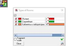
You can obtain a color scale (Fig. 10.2-63) and the coloring of floors into different colors depending on the type of room assigned to them for the models of the **FORUM** type for which the information on the types of rooms is specified.
