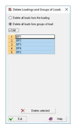
This operation enables to delete one or several loadings and groups of loads. Operations of deleting are performed in the respective dialog box (Fig. 8.5-2). Its list will contain the names of loadings or groups of loads depending on the selected radio button.
