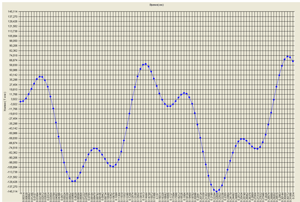
Graph of the variation of the bending moment M_2 in the cross-section of the beam with the attached mass subjected to the shear force, with time (tm-m)
