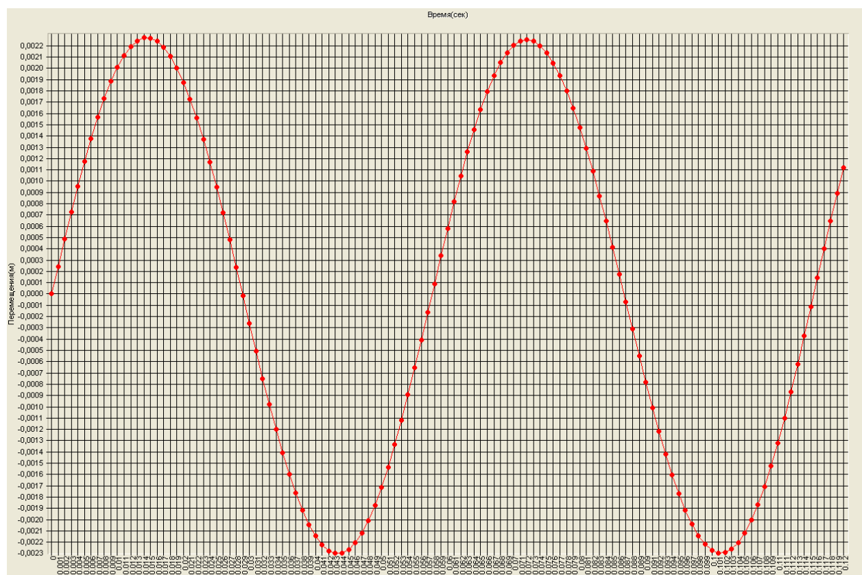
Graph of the variation of the transverse displacements of the nodal mass Z7 (closest to the end support) with time (m)
