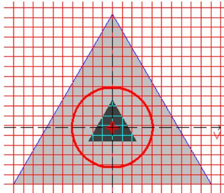
*Design model, coordinate and principal axes, center of mass, ellipse of inertia, core of the section*
