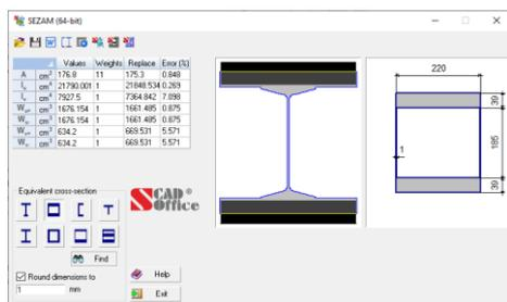
If a section has been selected as a file created by **Consul**, **Tonus** or **Section Builder**, the initial and equivalent sections are shown simultaneously in the window (Fig. 83), which allows to qualitatively assess their correspondence.
