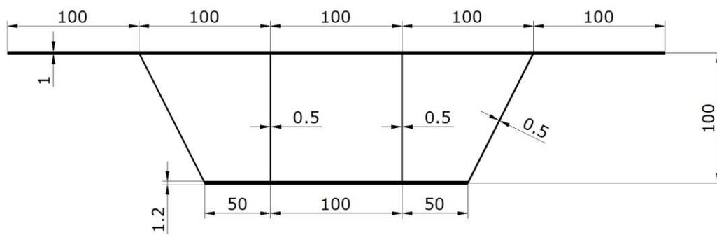
*Open-closed thin-walled section with sizes, cm*
