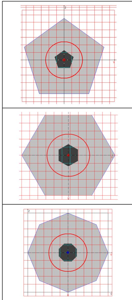
*Design model, coordinate and principal axes, center of mass, ellipse of inertia, core of the section*
