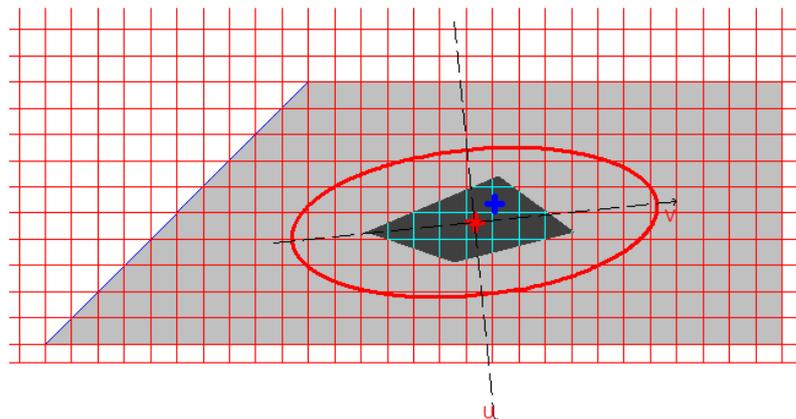
*Design model, coordinate and principal axes, center of mass, ellipse of inertia, core of the section*
