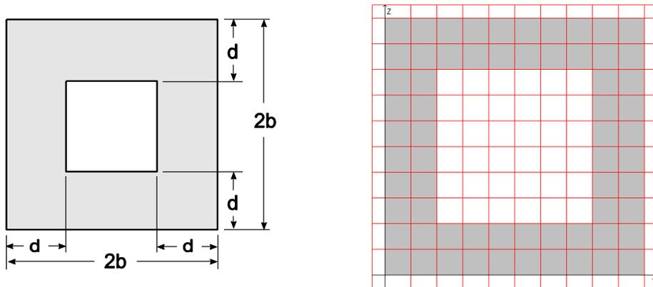
**Aim:** To check the accuracy of the torsional moment of inertia calculation for the cross-section of a rod with a hole.
