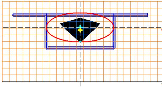
Design model, coordinate and principal axes, center of mass, ellipse of inertia, core of the section
