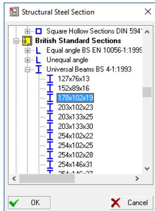
This command, which is invoked from the **File** menu, is used to select a section from the database, to modify it if necessary, and to examine its geometric properties. The section can be selected in the **Structural Steel Section** dialog box (Fig. 39).
