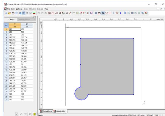
Figure 36. Create an arc on the contour:
