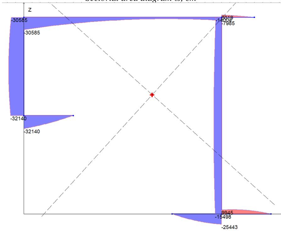
Sectorial static moment diagram  $S_{\omega}, \text{cm}^4$
