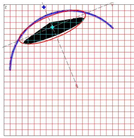
*Design model, coordinate and principal axes, center of mass, ellipse of inertia, core of the section*
