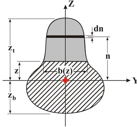
Figure 84. To defining of the section shear area
