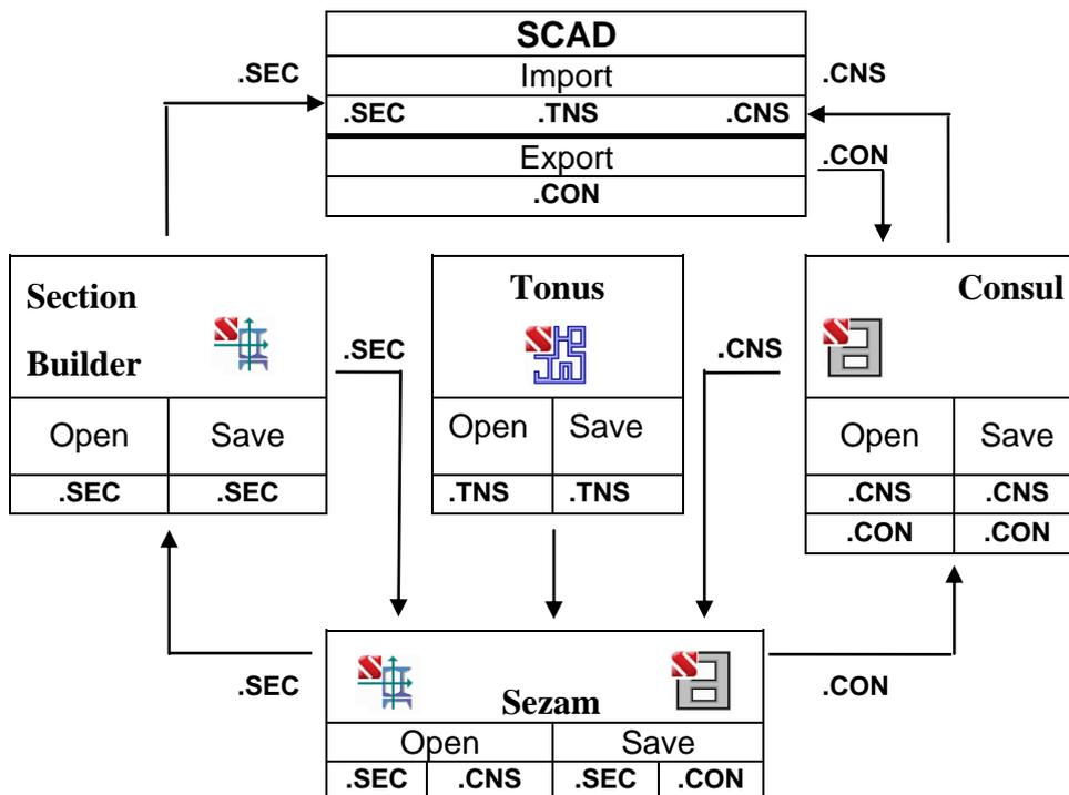
Figure 1. The diagram of interrelations between programs
