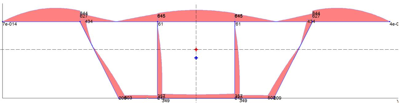
Diagram of the tangential stress module  $\tau_{\omega}$  for the value of the constrained torque  $M_{\omega} = 10^7$ ,  $kNcm$
