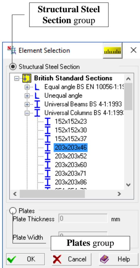
The **Element Selection** dialog box (Fig. 46) is invoked by clicking the **Select Element** button. This dialog box is used to select structural steel sections (**Structural Steel Section** group) and to specify the dimensions of plates (**Plates** group).
