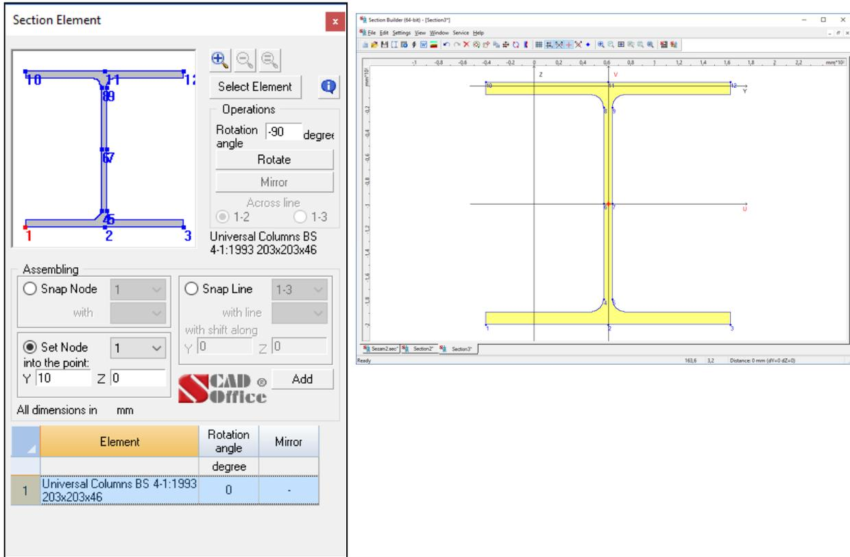
Figure 57. Result of creating the first section element
