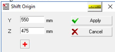
If you need to move the origin to the center of mass, click the red cross button. This will put the coordinates of the center into the respective text fields.
