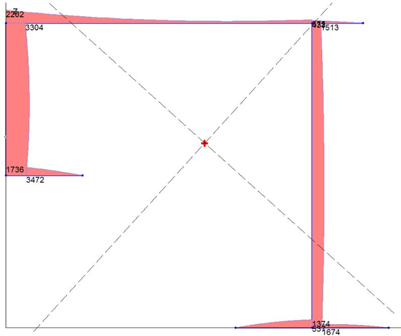
Diagram of the tangential stress module  $\tau_{\omega}$  for the value of the constrained torque  $M_{\omega} = 10^7$ , kNcm
