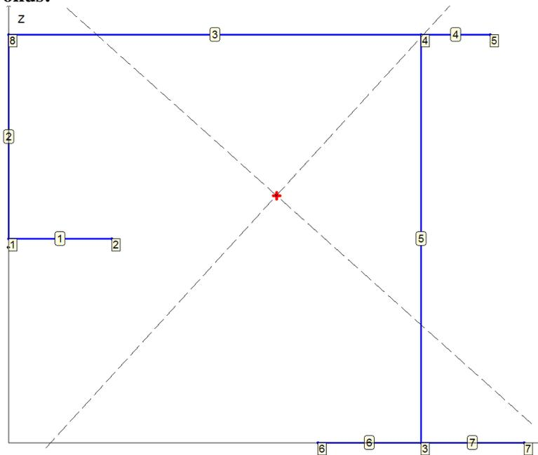
Numbering of vertices and strips, position of the mass center and shear center
