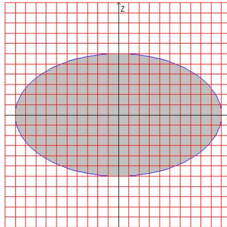
**Aim:** To check the accuracy of the geometric properties calculation for a solid elliptical cross-section of a rod.
