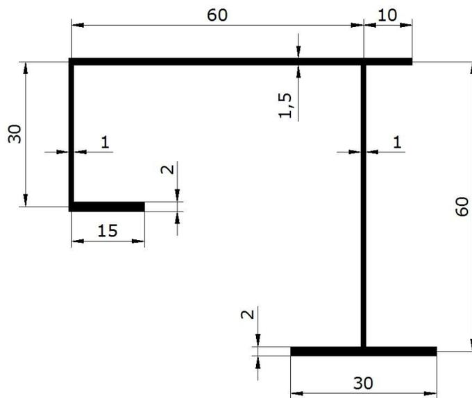
*Open thin-walled section with sizes, cm*
