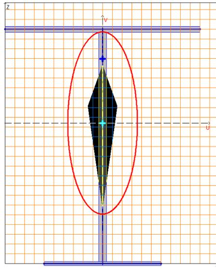
*Design model, coordinate and principal axes, center of mass, ellipse of inertia, core of the section*
