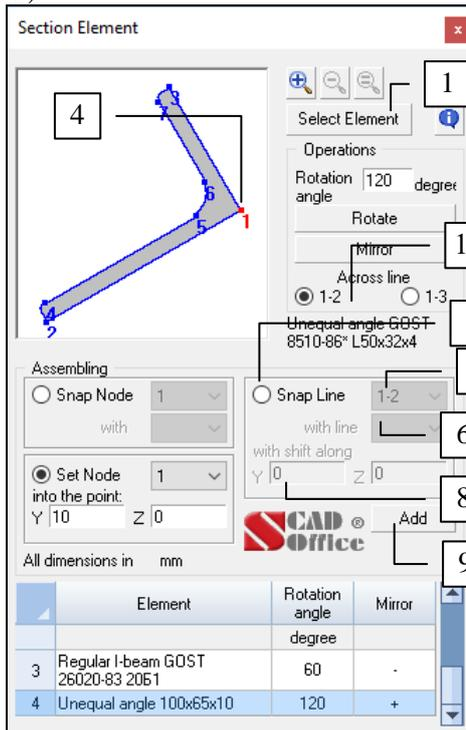
Figure 59. Joining by a line
