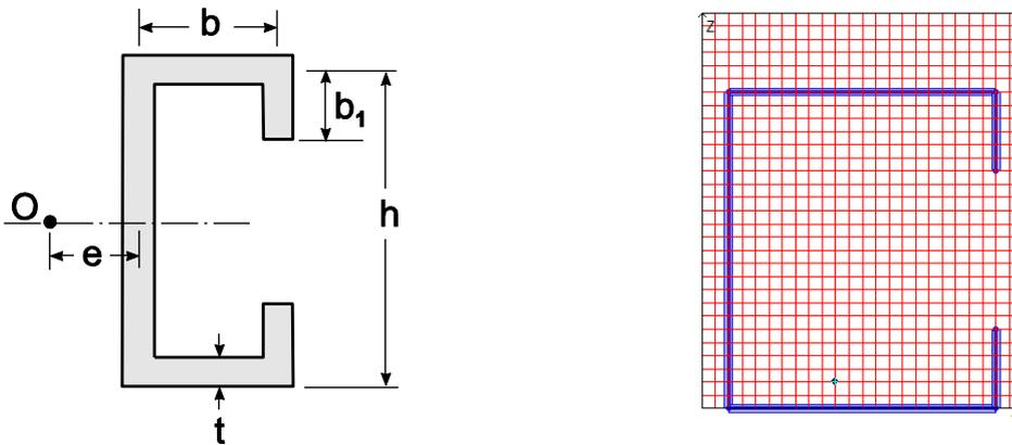
**Aim:** To check the accuracy of the geometric properties calculation for a C-shaped thin-walled section.
