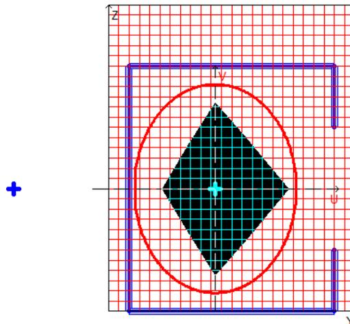
Design model, coordinate and principal axes, center of mass, ellipse of inertia, core of the section
