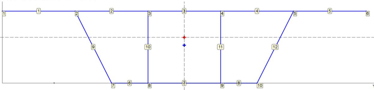
Numbering of vertices and strips, position of the mass center and shear center
