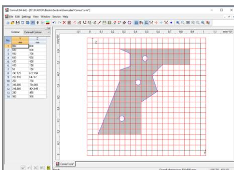
Figure 31. An example of a section with different internal contours
