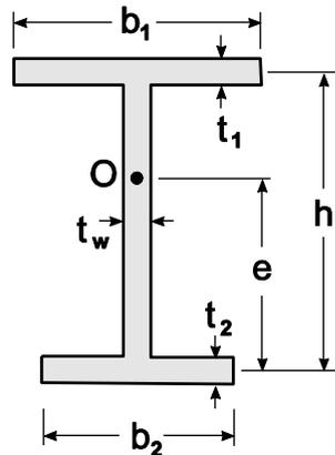
**Aim:** To check the accuracy of the geometric properties calculation for a thin-walled I-beam with unequal flanges.
