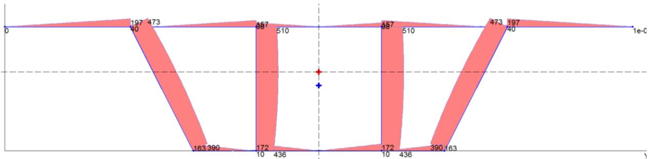
Diagram of the tangential stress module  $\tau_u$  for the value of the shear force  $Q_u = 10^5, \text{kN}$
