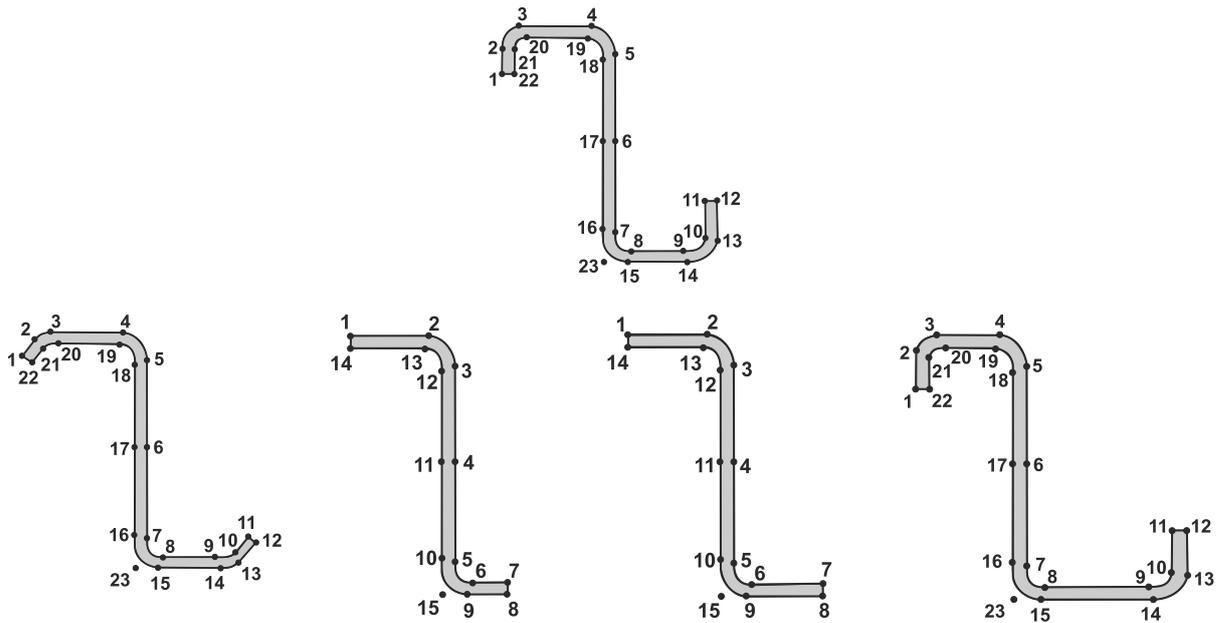
(base node is located in the center of the web)
