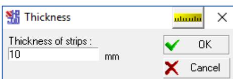
Clicking this button will open the **Thickness** dialog box (Fig. 69) the text field in which is used to specify a thickness for the section wall. The specified value will be assigned by default to all newly added strips.
