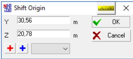
If you need to move the origin to the center of mass, to the center of shear or to a particular vertex, click the red cross button, blue cross button or select the number of the vertex from the drop-down list, respectively. This will put the coordinates into the respective text fields.
