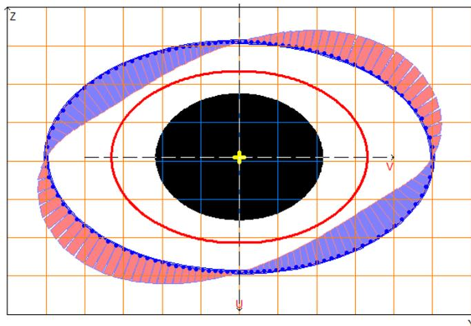
Design model, principal axes, center of mass, ellipse of inertia, core of the section, sectorial coordinate diagrams
