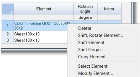
Double-clicking on a row of the table highlights it and selects the corresponding element of the section (it is highlighted in the **Section Builder** window).
