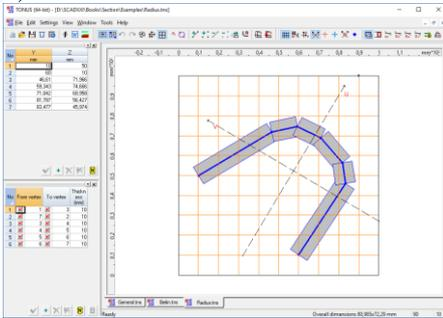
Depending on whether this button is pressed or depressed, the work area will display either a whole section (if the button is pressed) or just a contour of it, i.e., the center lines of the strips (Figs. 75, a and 75, b respectively).
