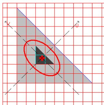
*Design model, coordinate and principal axes, center of mass, ellipse of inertia, core of the section*
