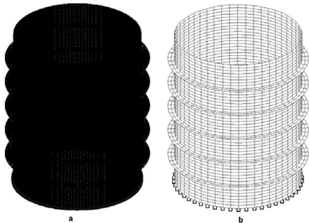
Fig. 4. Ribbed shell with discrete welded connection. a – computational model with fine mesh, b – model with a coarse mesh
