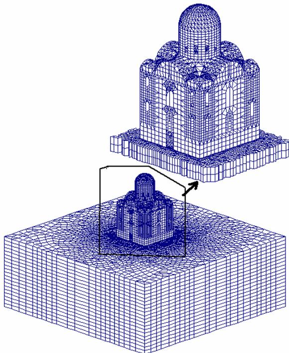
Fig. 5 Structure – soil interaction problem
