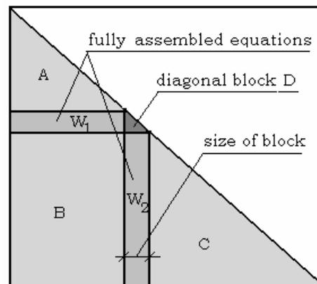
Fig. 2. Block factoring of stiffness matrix
